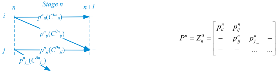
Fig. 4. Graph of the possible transitions between states i, j and k of stage n for a policy decision x_n=0
