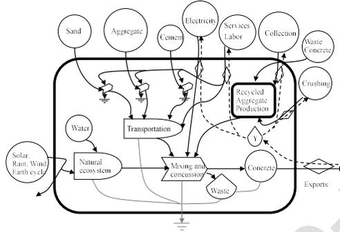
(3) Energy flow of fly ash concrete (FAC) production
