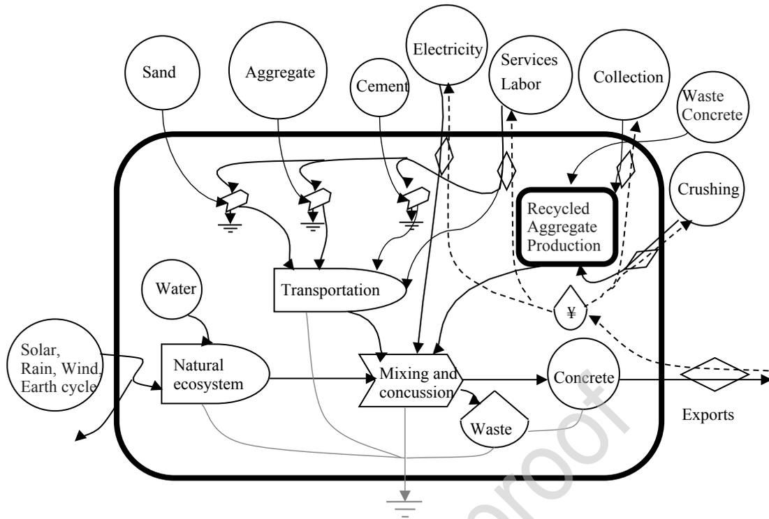
Figure 3 Energy flow of recycled aggregate concrete (RAC) production
