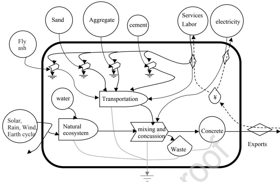
Figure 4 Energy flow of fly ash concrete (FAC) production
