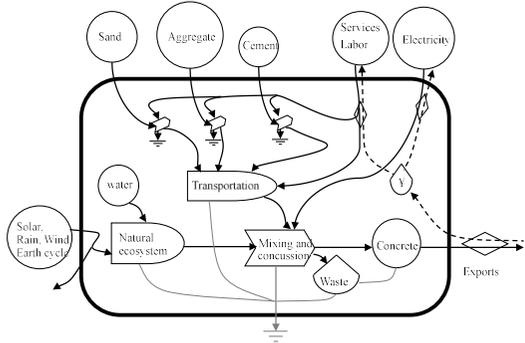
(2) Energy flow of recycled aggregate concrete (RAC) production
