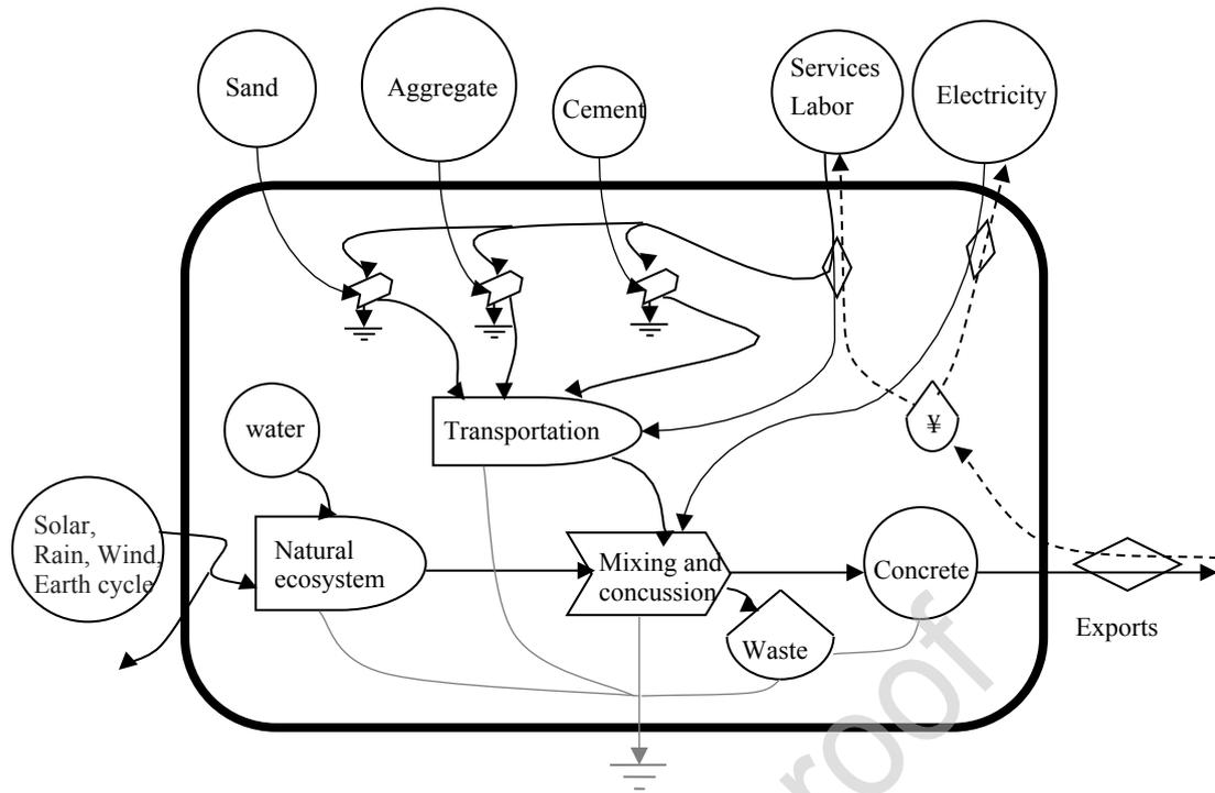
Figure 2 Energy flow of traditional concrete production
