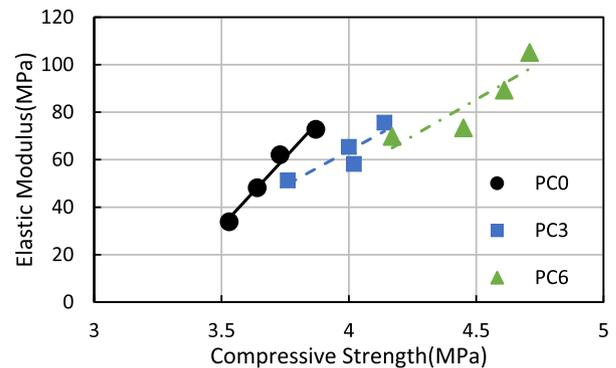
Fig. 18. Relationship between compressive strength and elastic modulus of plastic concrete mixture designs.
