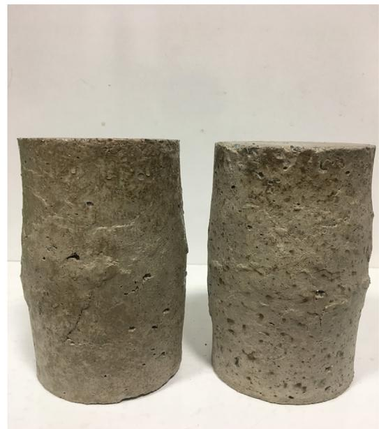
Fig. 10. Failure mode of plastic concrete under triaxial compressive strength test.
