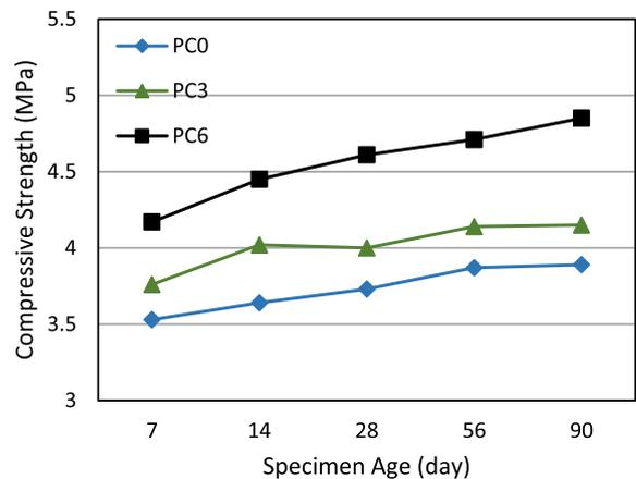
Fig. 7. Compressive strength for different mixture design and different specimen age.
