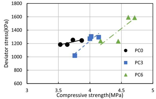
Fig. 17. Relationship between compressive strength and deviatoric stress of plastic concrete mixture designs.
