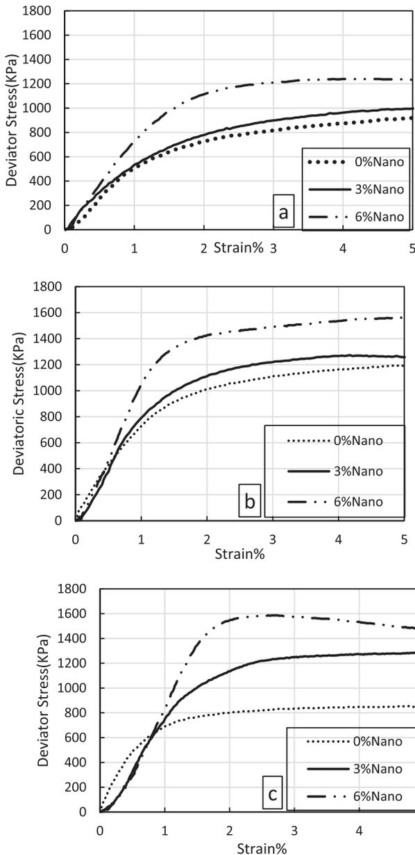
Fig. 9. Effect of nano silica content on peak stress in specimen with (a) 7 days age, (b) 28 days age and (c) 56 days age.
