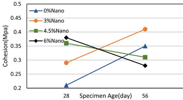
Fig. 15. Effect of nano silica on cohesion parameter with different specimen age.
