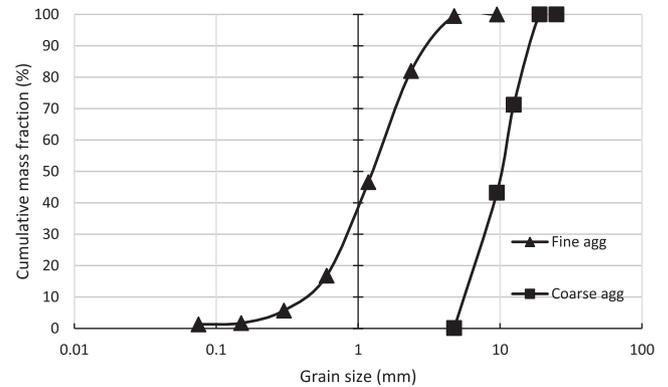
**Fig. 1.** Particle size distribution (PSD) curves of fine and coarse aggregates.
