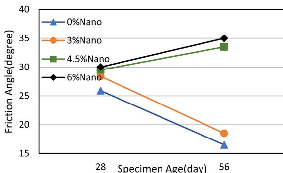
Fig. 16. Effect of nano silica on friction angle parameter with different specimen age in plastic concrete.
