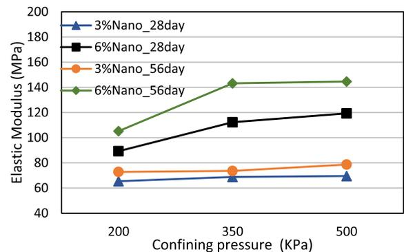
Fig. 14. Effect of confining pressure on elastic modulus of plastic concrete with nano silica (28 and 56 days specimen age).
