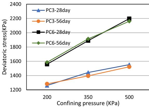
Fig. 12. Effect of different confining pressure on peak stress with different mixture design.
