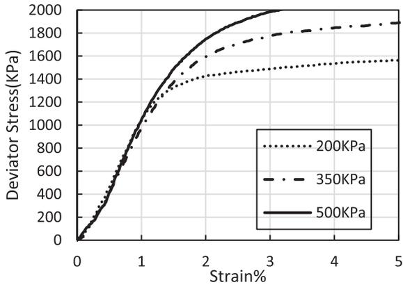
Fig. 11. Effect of confining pressure on peak stress on PC6 specimen mixture design and 28 days specimen age.
