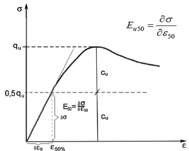
Fig. 4. Elasticity modulus ( $E_{u50}$ ) determination from nonlinear stress–strain relationship.
