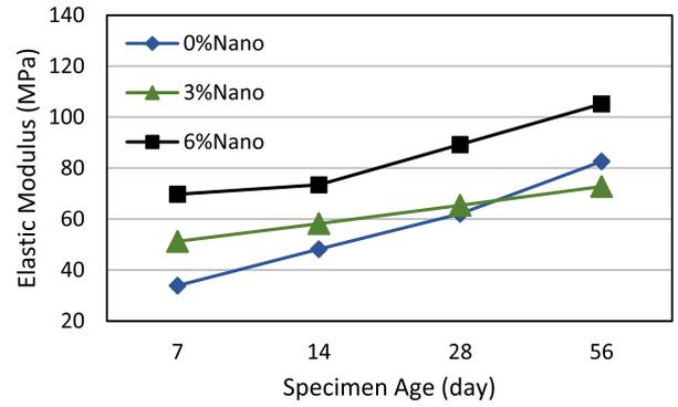
Fig. 13. Effect of nano silica and specimen age on elastic modulus.
