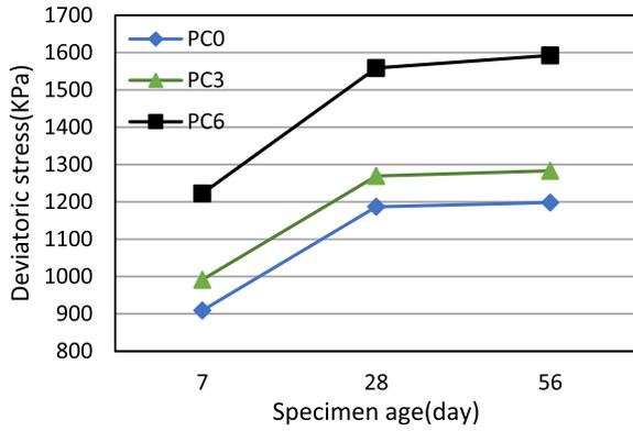
Fig. 8. Deviatoric stress for different mixture design and different specimen age.
