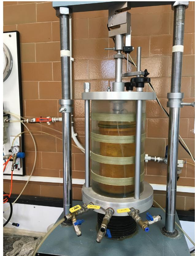
Fig. 3. Triaxial apparatus during testing.
