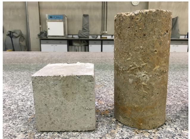
**Fig. 2.** Cylindrical and cubic specimen.
