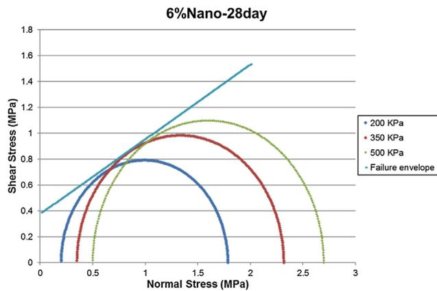
Fig. 5. Mohr circles for PC6 specimen at age of 28 days.
