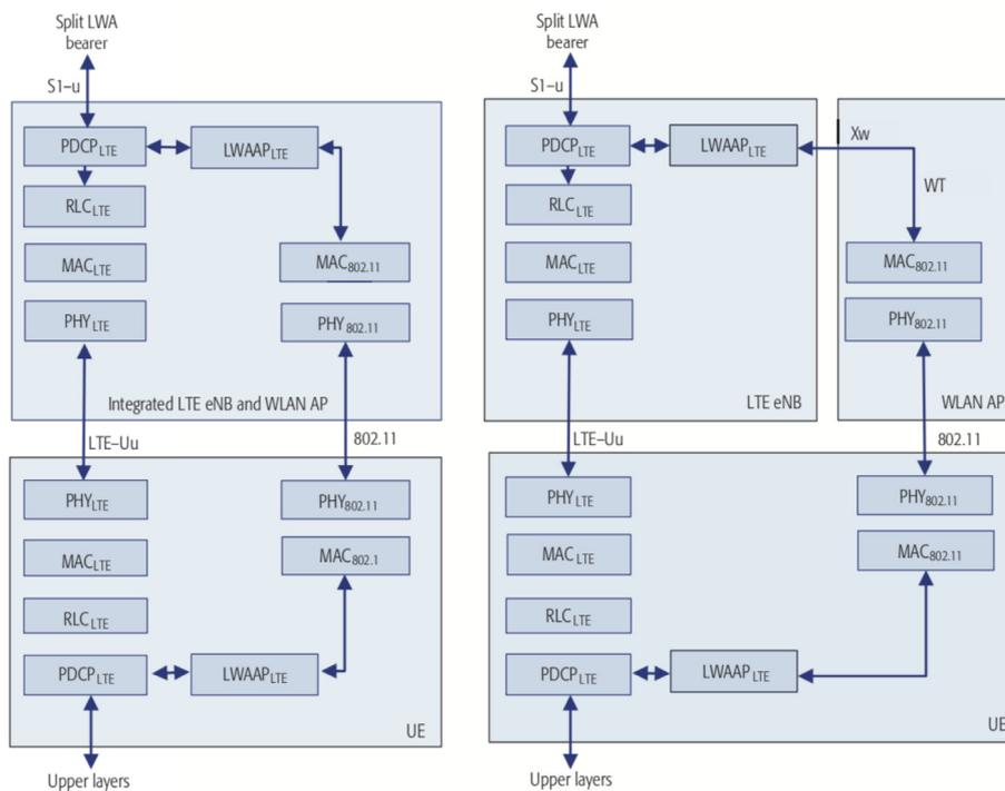
Fig. 6. The LWA architecture providing the options of an integrated access point or an external one [47].
