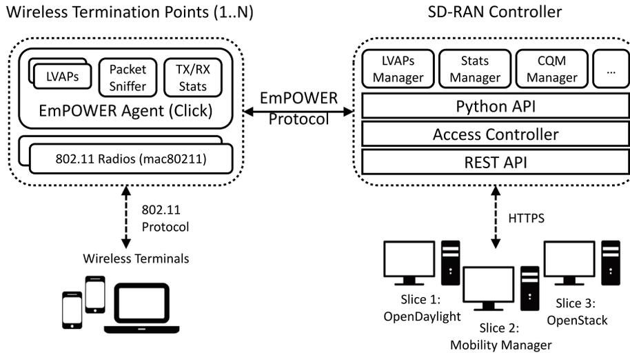
Fig. 5. The 5G-EmPOWER architecture as an example of SDN in wireless networks [46].
