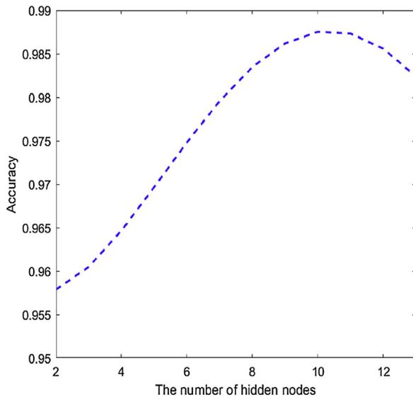
Fig. 8. Accuracy of different hidden nodes on the experimental data set in ANN.
