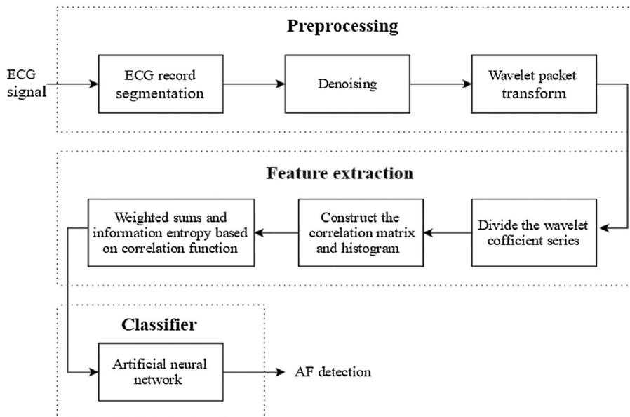
Fig. 3. The framework of the proposed algorithm for AF detection.
