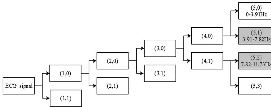
Fig. 1. A part of the tree-structure of a 5-level wavelet packet transform.
