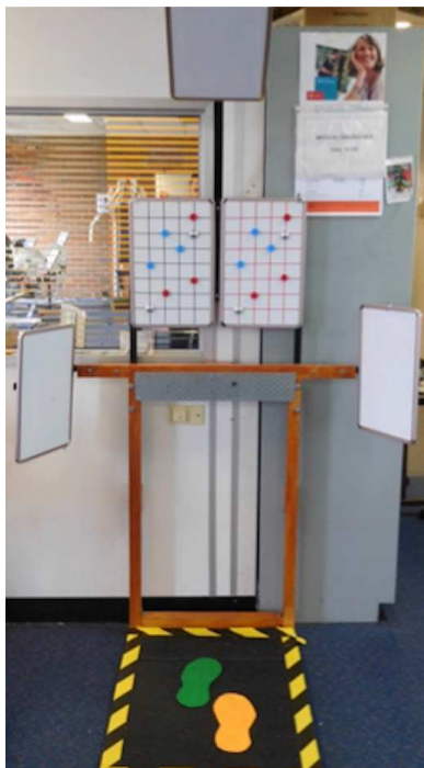
Figure 3 – Static balance dual-task apparatus (colour) - The custom-made apparatus, affectionately named 'Humphre' - consists of coloured button magnets, and magnetic whiteboards laterally, in front, and above the participant to allow completion of physical and cognitive dual-task. A grab bar in front of the participant provides additional support during the movement.
