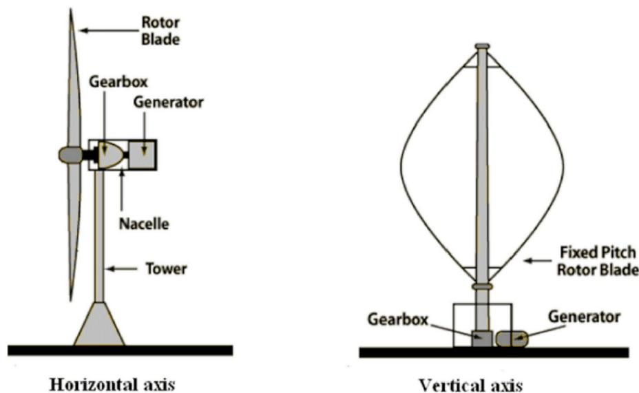
Fig. 3. Typical horizontal and vertical axis wind turbines (after [2]).
