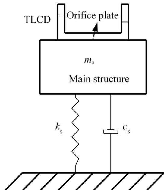
Fig. 15. A main structure-TLCD system.
