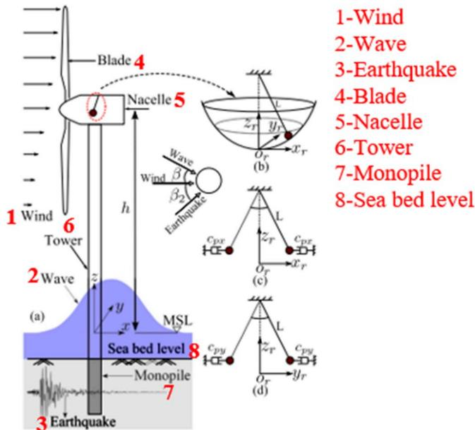
Fig. 14. 3D pendulum TMD proposed by Sun and Jahangiri (after [41–43]).
