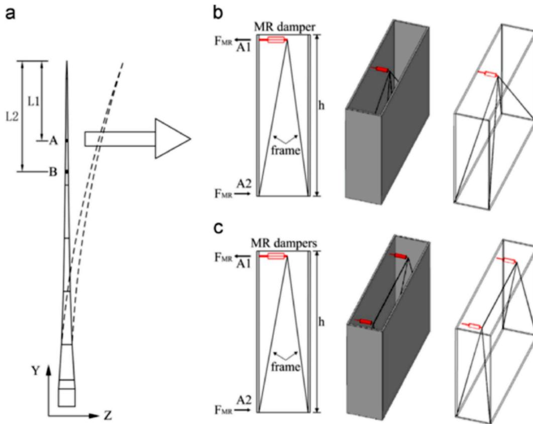
Fig. 26. Configuration of blade with MR damper (after [108]).
