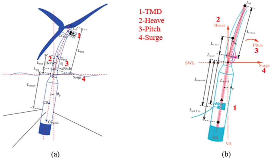
Fig. 11. Using TMD to control the vibration of floating offshore wind turbines with TMD installed (a) in the nacelle (after [29]) and in the spar-buoy platform (after [30]).
