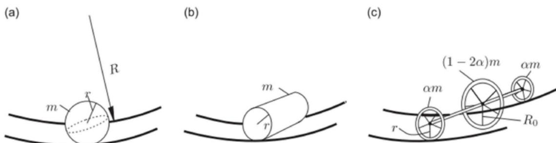
Fig. 23. Possible layouts of roller damper (after [98]).
