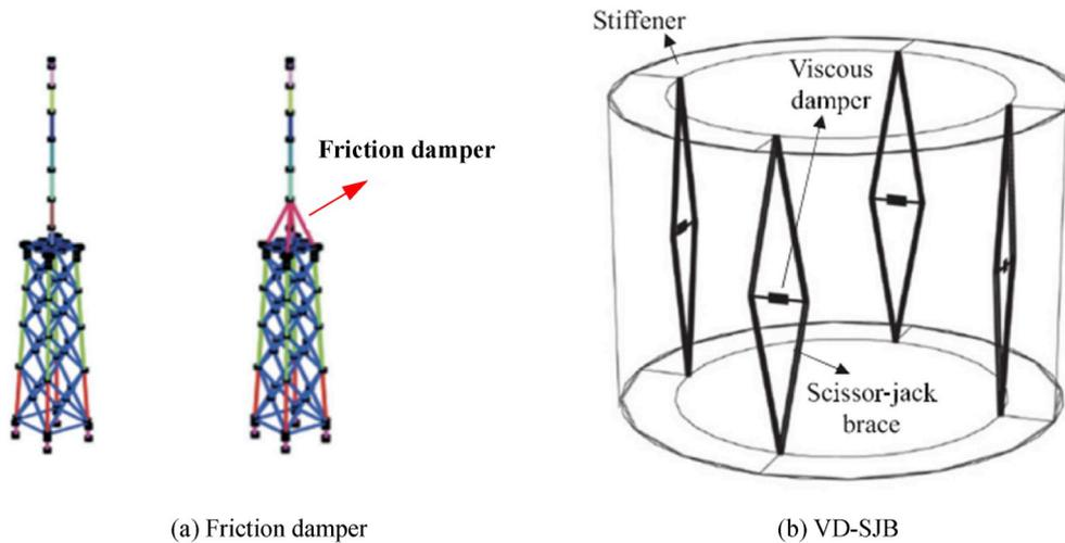
Fig. 18. Offshore wind turbine without and with (a) friction damper (after [63]) and (b) VD-SJB (after [64]).
