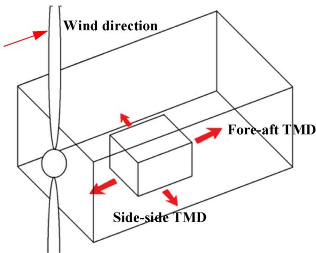
Fig. 7. Fore-aft and side-to-side TMDs in a nacelle (after [23]).
