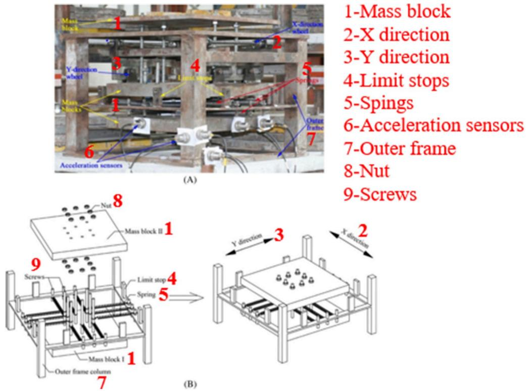
Fig. 13. Two linear TMDs installed in the nacelle (after [40]).
