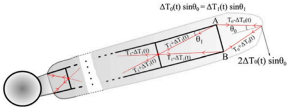
Fig. 24. Active control of the blade in-plane vibration using active tendons (after [102–104]).
