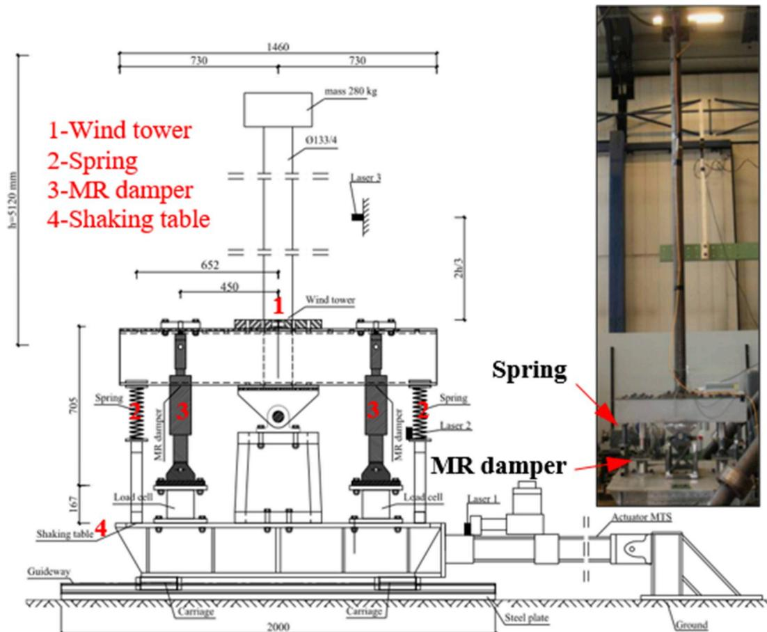
Fig. 21. Experimental setup of a wind turbine tower with MR dampers (after [78]).
