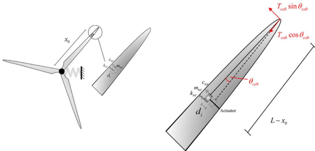
Fig. 25. Cable connected ATMD inside the blade (after [106]).
