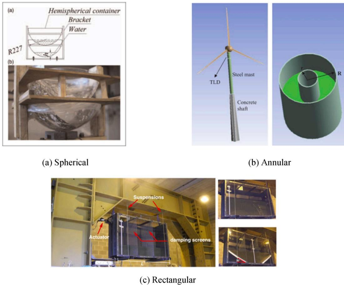
Fig. 17. Different geometrical types of TLDs (after [58,59,61,62]).
