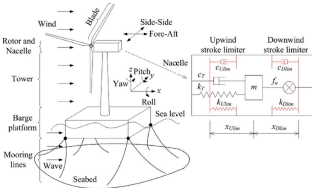
Fig. 20. Barge-type floating offshore wind turbine with a stroke-limited ATMD (after [74]).
