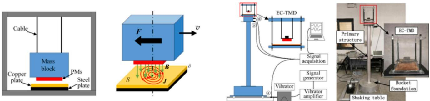
Fig. 8. Damping mechanics and experimental layouts of the EC-TMD system (after [24]).
