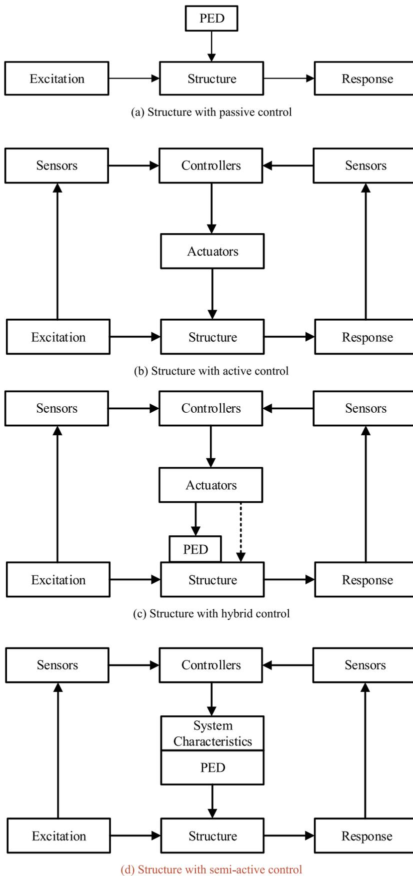
Fig. 5. Working mechanisms of different vibration control methods (after [10]).
