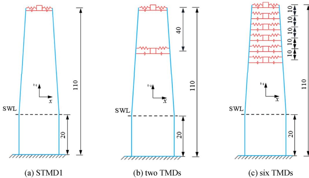
Fig. 9. Three different TMD arrangements adopted in Ref. [25].
