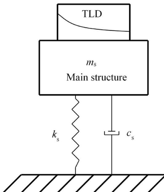
Fig. 16. A main structure-TLD system.
