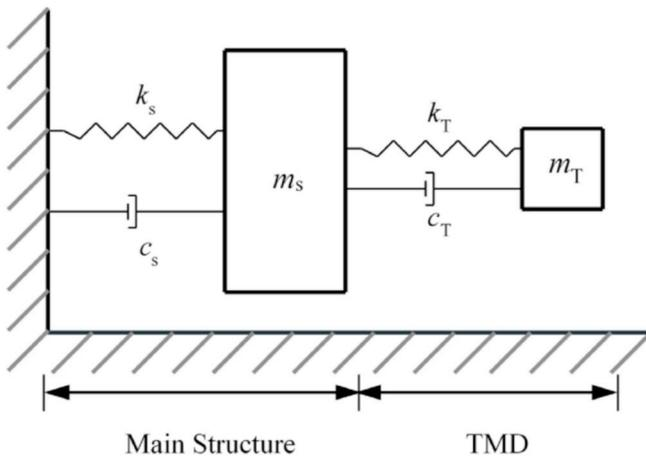
Fig. 6. A main structure-TMD system.
