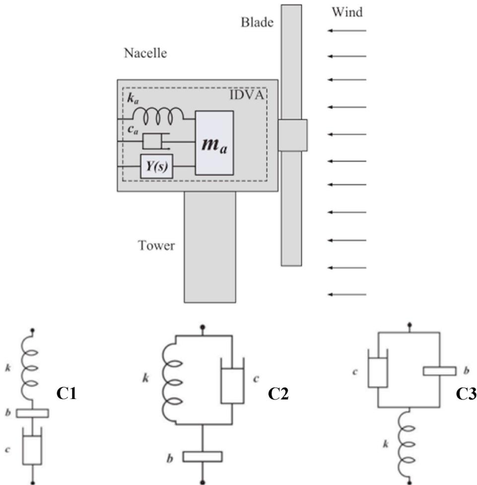
Fig. 12. Schematic of the inerter-based TMD system and three configurations for  $Y(s)$  (after [35]).
