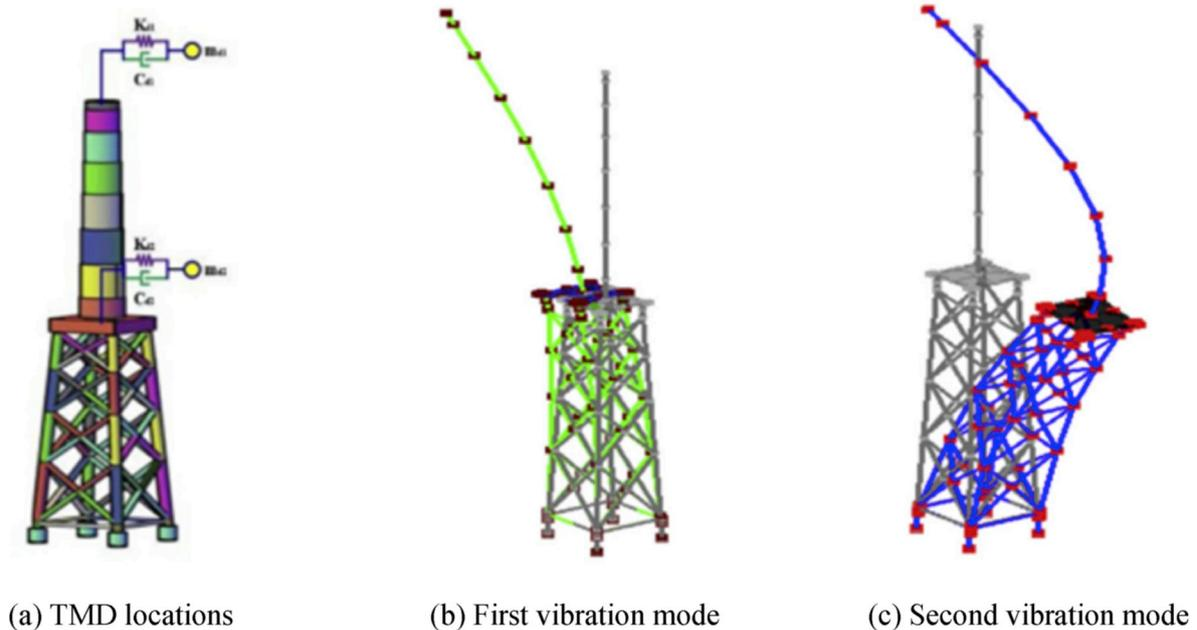
Fig. 10. TMD arrangement and vibration modes of a jacket-support offshore wind turbine (after [26]).
