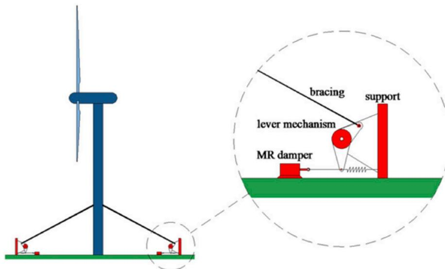
Fig. 22. Outer bracing MR dampers connected to the wind turbine tower (after [79]).
