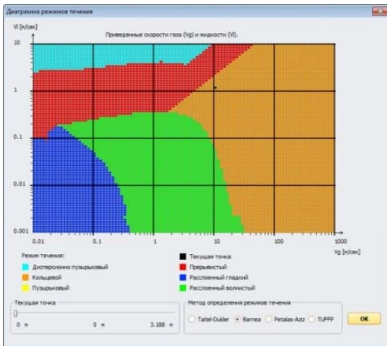
Fig. 5. Design regimes of two-phase flow in vertical channels
