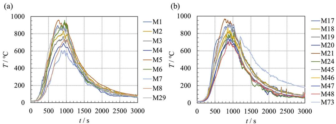
Fig. 12. Member temperature-time curves obtained in the test.
