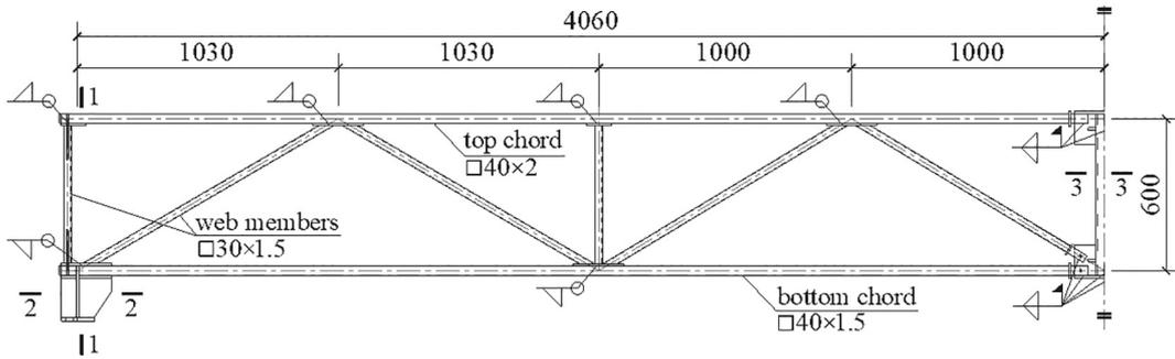
Fig. 10. Details of the main trusses [9].
