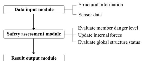
Fig. 6. System modules and functions.
