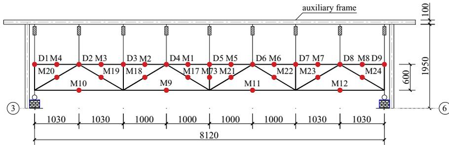
Fig. 11. Sensors for structural components.
