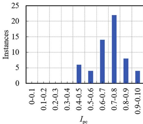
Fig. 5. Summary of collapse index distribution of steel truss.
