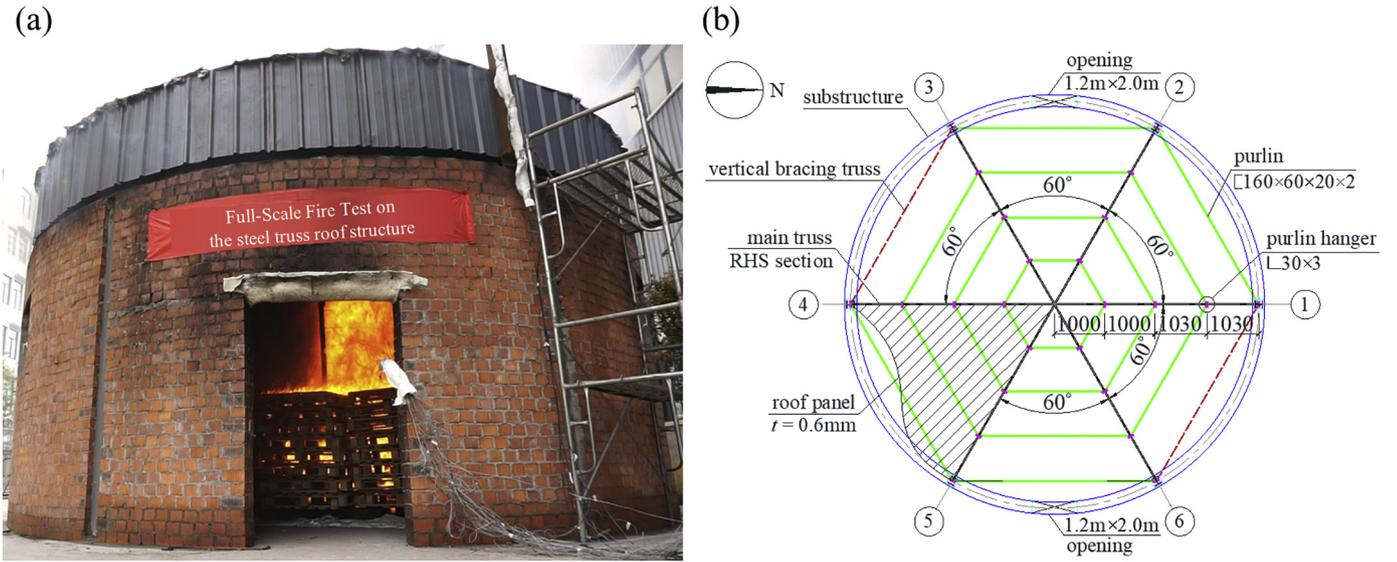
Fig. 9. Overall configuration of the test model [9]. (a) Overview. (b) Planar view.
