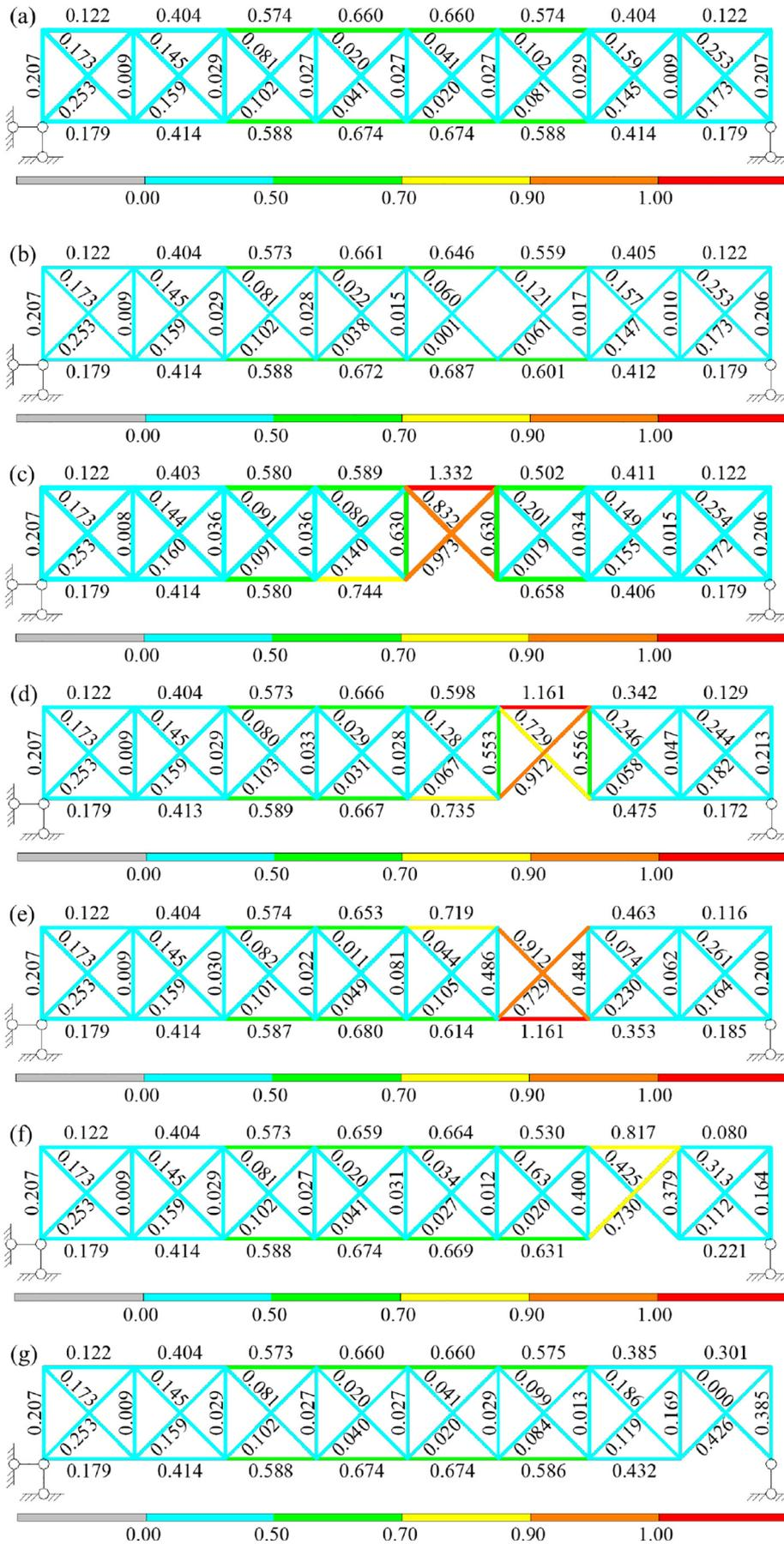
Fig. 4. The stress ratio of the structure after the demolition of some components. (a) Original structure. (b) No. 6. (c) No. 18. (d) No. 20. (e) No. 21. (f) No. 22. (g) No. 24. (h) No. 30. (i) No. 31. (j) No. 32. (k) No. 33.
