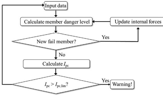
Fig. 7. Design of the module of safety assessment.
