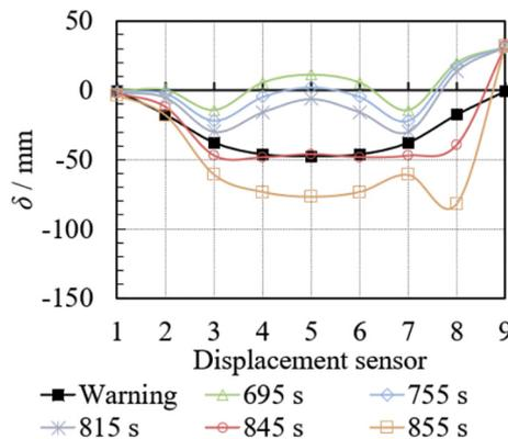
Fig. 15. Comparison of the predicted structural response and the test results.
