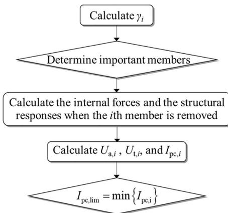
Fig. 2. Calculation procedures of collapse index limit value.
