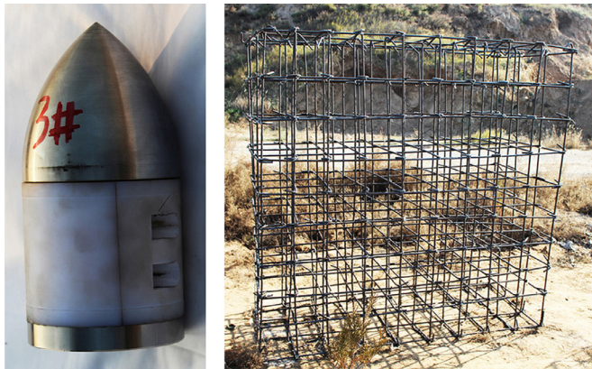
(a) Experimental projectile (b) Layout of the reinforcing bars
