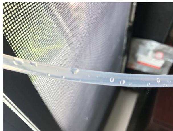
Fig. 6. Water carried out by the outlet gas during the reaction of oxygen carrier regeneration.
