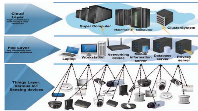
Fig. 1. Three tiers IoT, Fog and Cloud Architecture [11]
