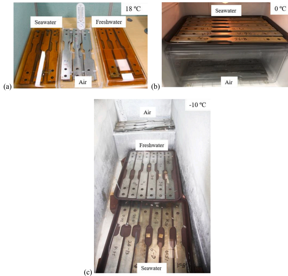
Fig. 3. Test specimens kept in dry or water-immersed condition in seawater, freshwater and air at (a) 18 °C, (b) 0 °C and (c) -10 °C.
