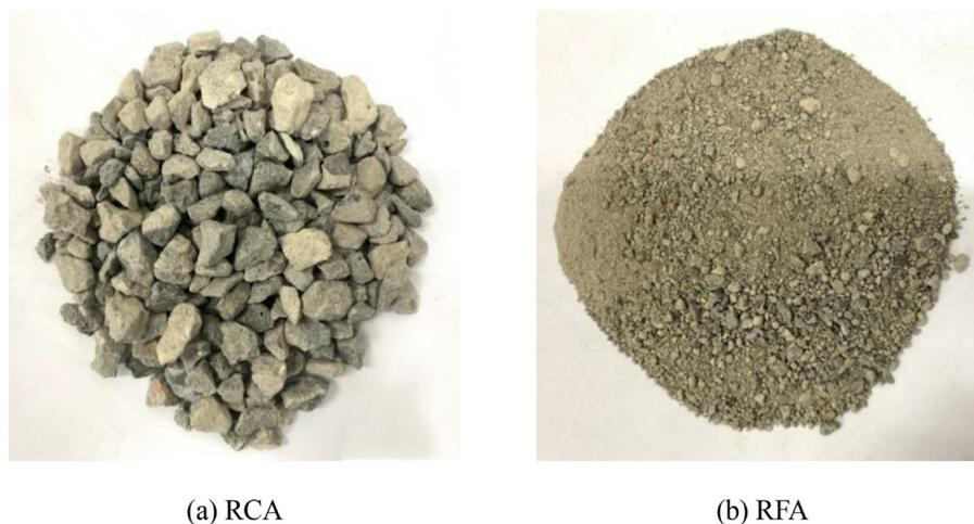
Fig. 1. Recycled aggregates: a) RCA, b) RFA.
