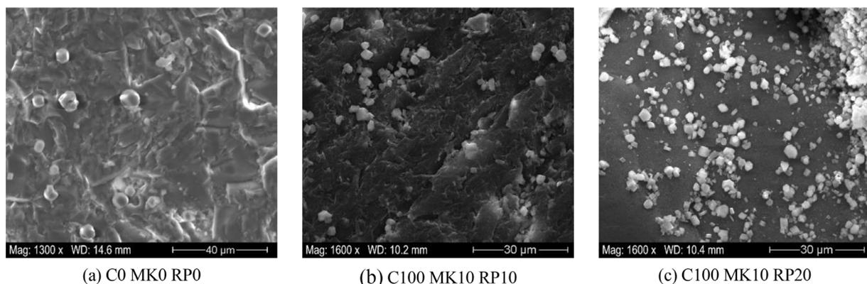
Fig. 14. Microstructure of the surface hydration of the concrete.
