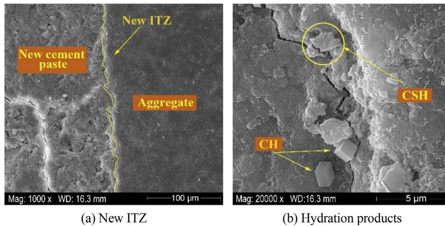
Fig. 13. Microstructure of the new ITZ in M2 (C25 MK10 RP10).
