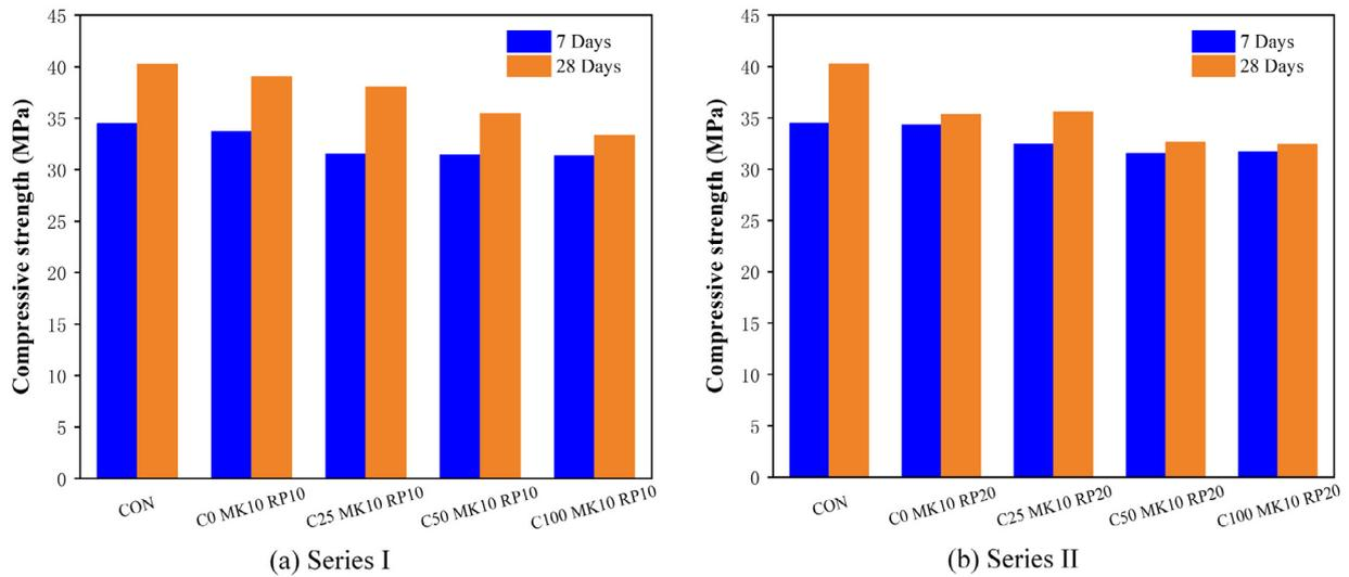
Fig. 9. Compressive strength of SCC mixes with different WCRMs content.
