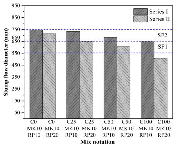
(b) Effect of RP content on the slump flow diameter
