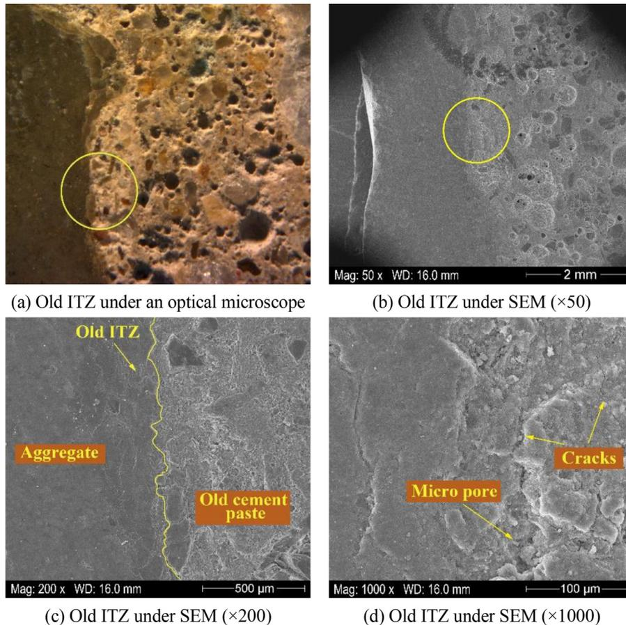
Fig. 12. Microstructure of the old ITZ in M4 (C100 MK10 RP10).
