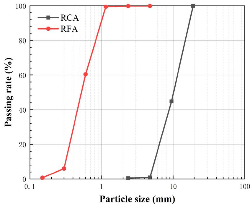
Fig. 2. Sieve analysis curves of the RCA and RFA.
