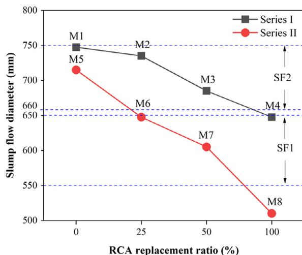
(a) Effect of RCA content on the slump flow diameter
