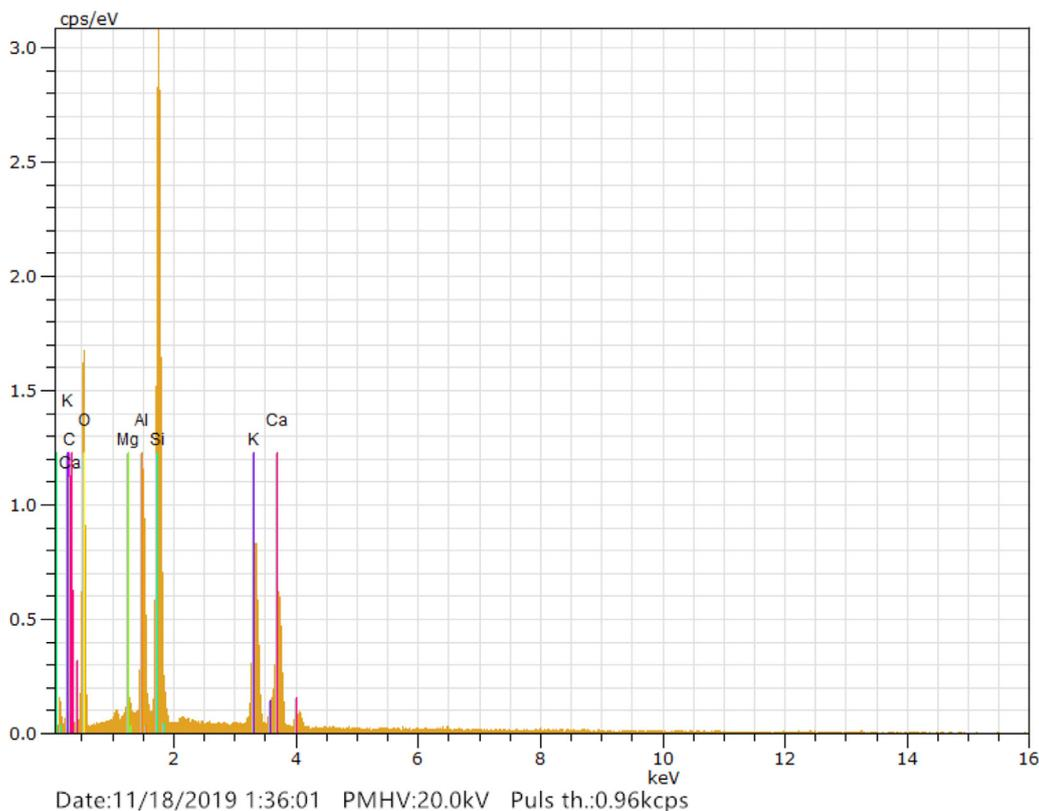
Fig. 15. EDS elemental analysis on the surface of M8.
