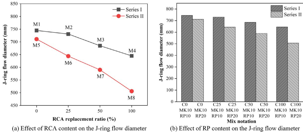
Fig. 8. J-ring flow diameter of the SCC mixes.
