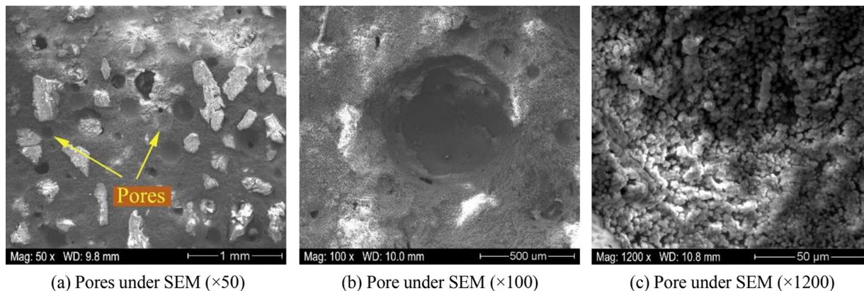
Fig. 16. Pores on the surface of M8 (C100 MK10 RP20).
