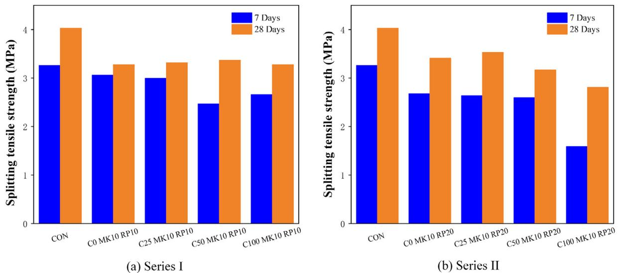
Fig. 10. Splitting tensile strength of SCC mixes with different WCRMs content.
