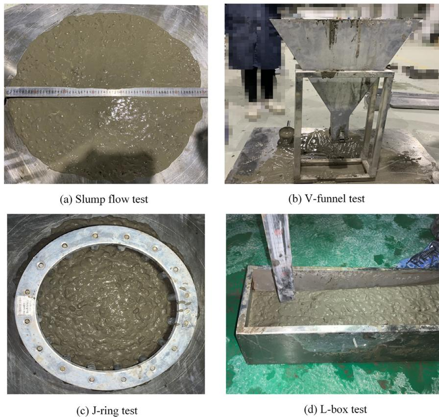
Fig. 3. Processes for the workability property tests.
