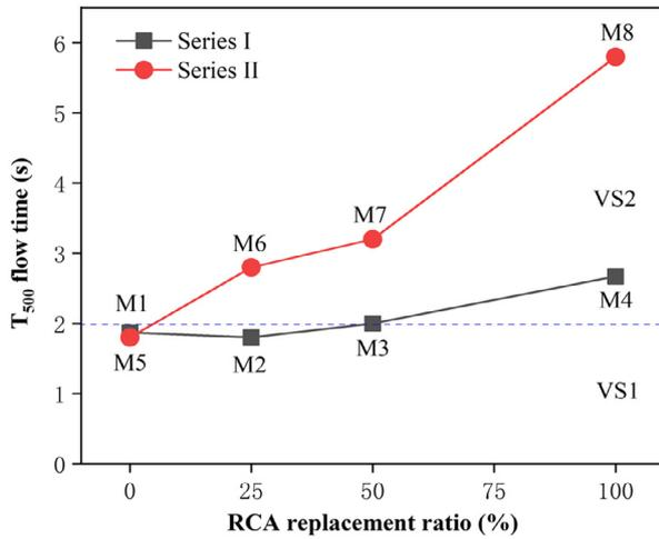
(a) Effect of RCA content on  $T_{500}$  flow time
