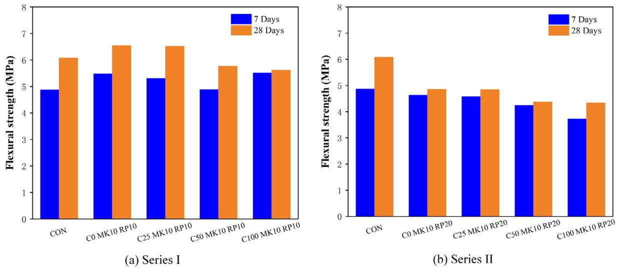
Fig. 11. Flexural strength of SCC mixes with different WCRMs content.
