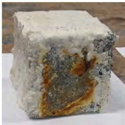
Fig. 11. Picture (left) showing the froth formation around the control sample kept in 3.5% sulfuric acid solution for 28 days and the graph on the right shows the XRD diffractogram of the froth along with its XRF analysis.
