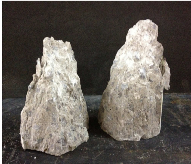
1 2 Figure 13. Comparison of the concrete fracture surface obtained at moderate (right) and high frequency (left).
