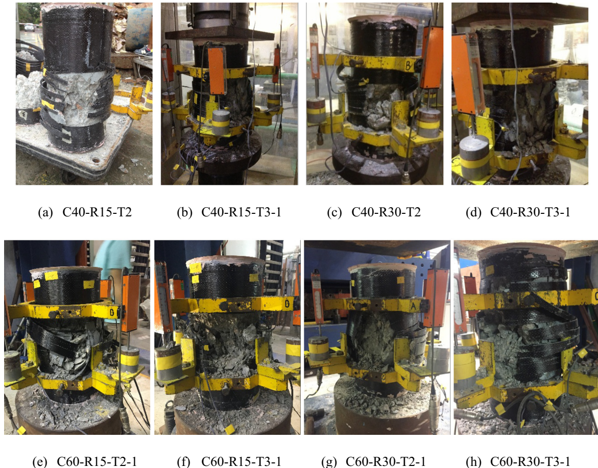
Fig. 6. FCCC columns after test.
