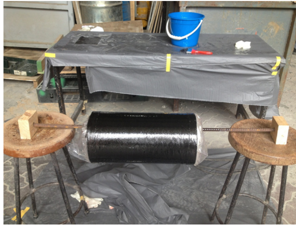
(b) Wrapping of a carbon fiber sheet
