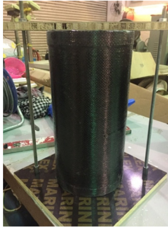
(c) CFRP tube after curing
