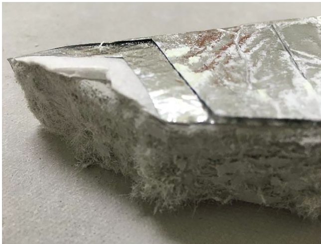
Fig. 3a. VIP core with the layers (non-woven fabric and (silvery) laminate).
