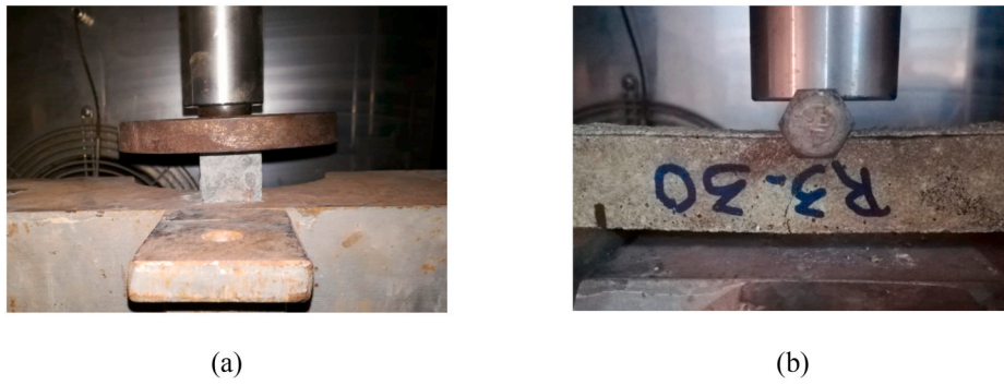
Fig. 3. Mechanical tests a) compression and b) flexural.
