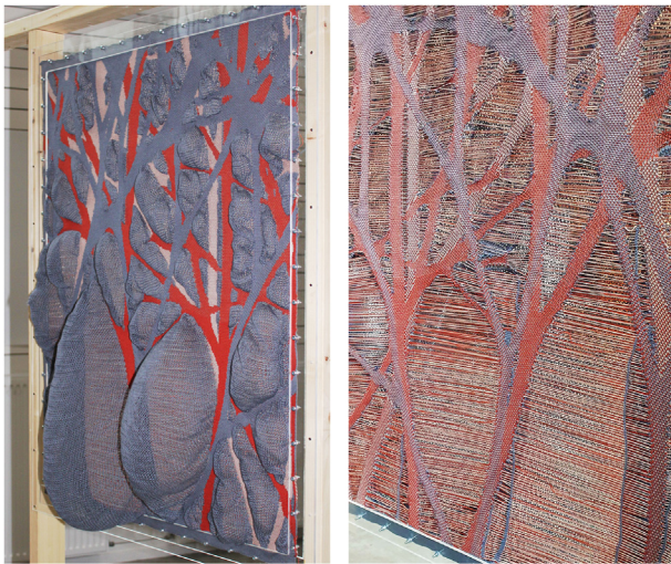
Fig. 25 The drop-stitch pattern combined with three-colour jacquard. Left: the right side of the piece. Right: the purl side of the piece in detail.
