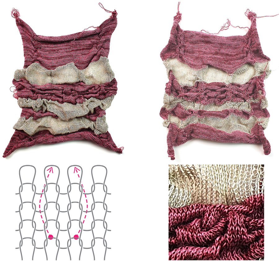
Fig. 12 Top: sample produced using the hanging stitches technique, seen from the right, and purl side. Yarns: wool 28/2 \times 3 in two shades of pink, stitch length 5, and uncoloured linen, stitch length 7. Knitted on 80 needles. Bottom: illustration of the knitting technique and a close-up. Note, this sample was fixed at a set of points to keep edges from curling in.
