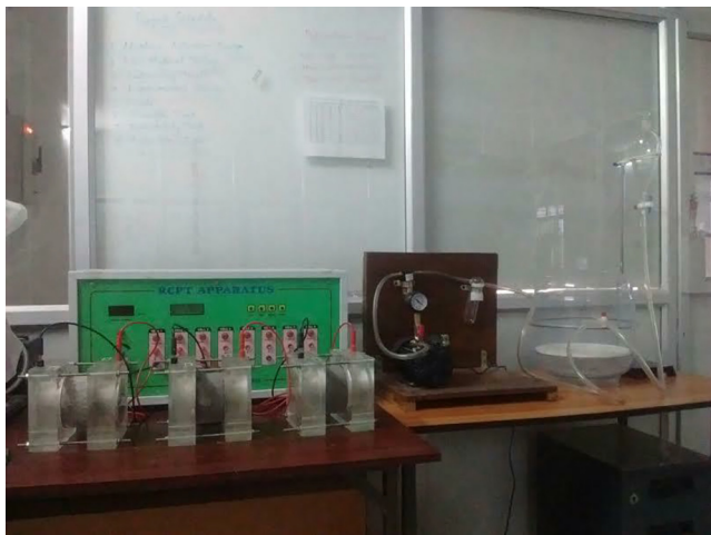
Fig. 12. Rapid Chloride Penetration Set up.
