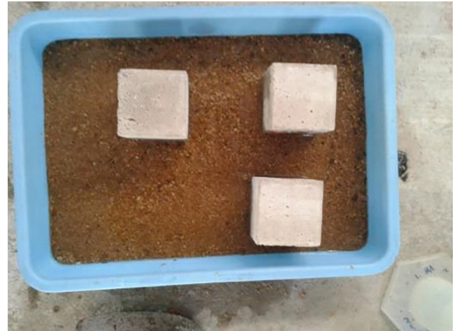
Fig. 10. Sorptivity Test set up.
