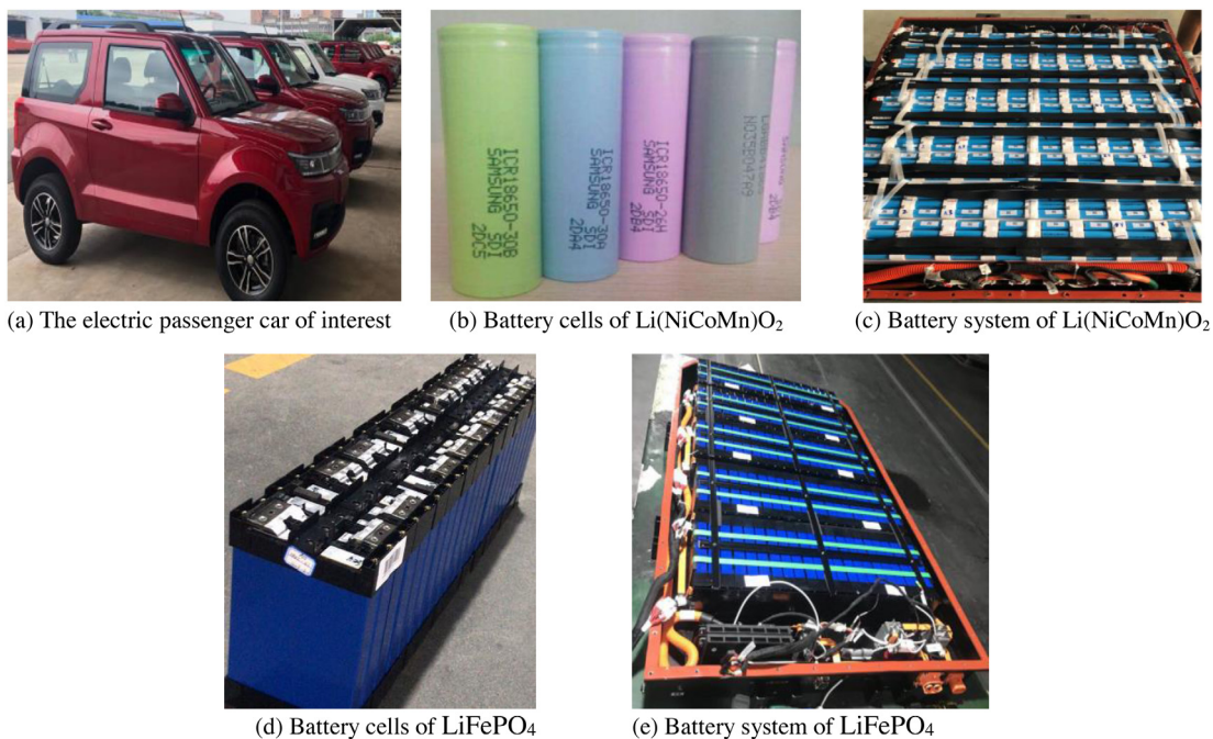
Fig. 2. Electric passenger car and its battery system.
