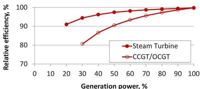
Fig. 4. Estimated relative power plant efficiency at various generation outputs.
