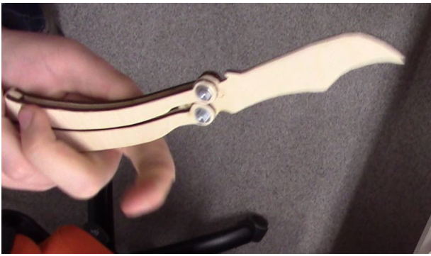
Fig. 2. Butterfly knife with the design originating from a video game, made with a laser cutter.
