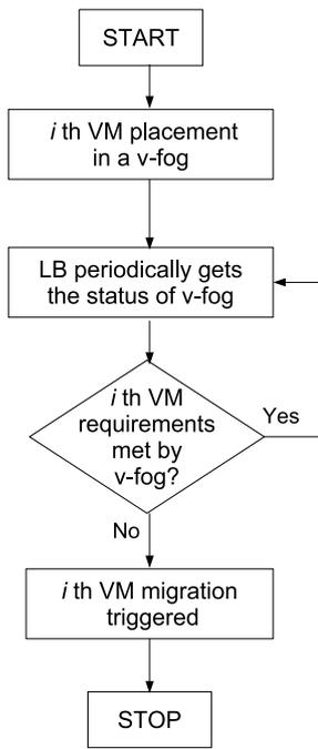
Fig. 6. Flowchart for VM migration trigger algorithm in MB.
