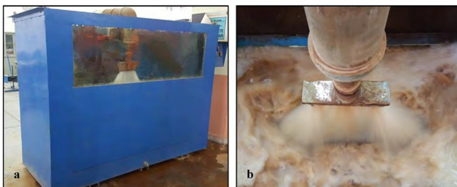
Fig. 1. (a) Water –Jet test Machine; (b) Jet.
