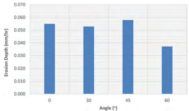
Fig. 8. Erosion depth for different angles C25.
