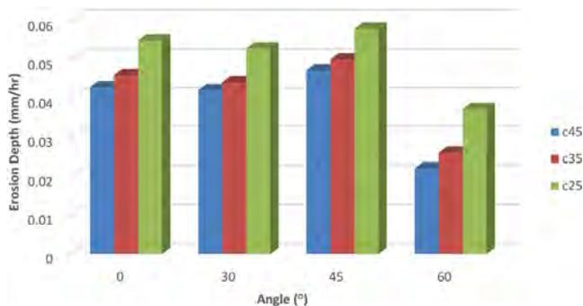
**Fig. 9.** Erosion depth for different compressive strength.
