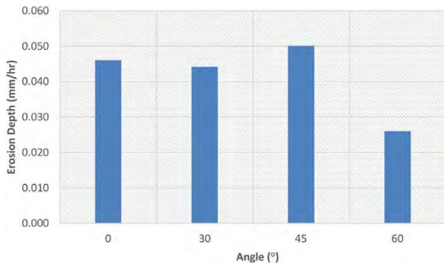
Fig. 7. Erosion depth for different angles C35.
