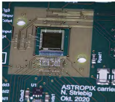
(b) Picture of the AstroPix V1 detector on a carrier board.
