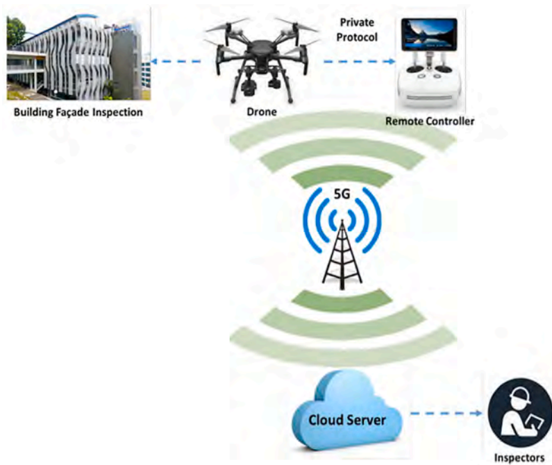
Fig. 17. Workflow of a 5G-powered Façade Inspection System using AI and Drones
