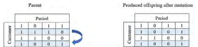
Fig. 6. The mutation operation on matrix chromosome.
