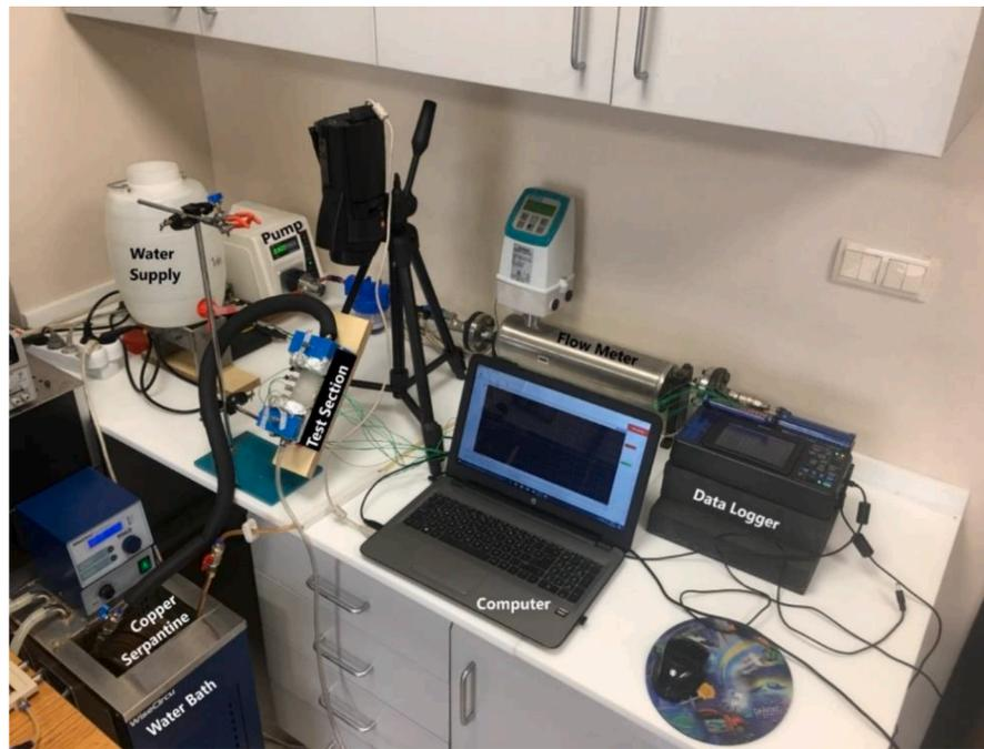
Fig. 2. Actual photograph of the experimental setup.
