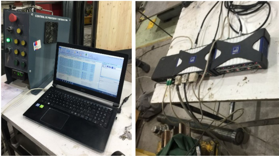
Fig. 13 Data acquisition equipment connected to LVDT and load cell
