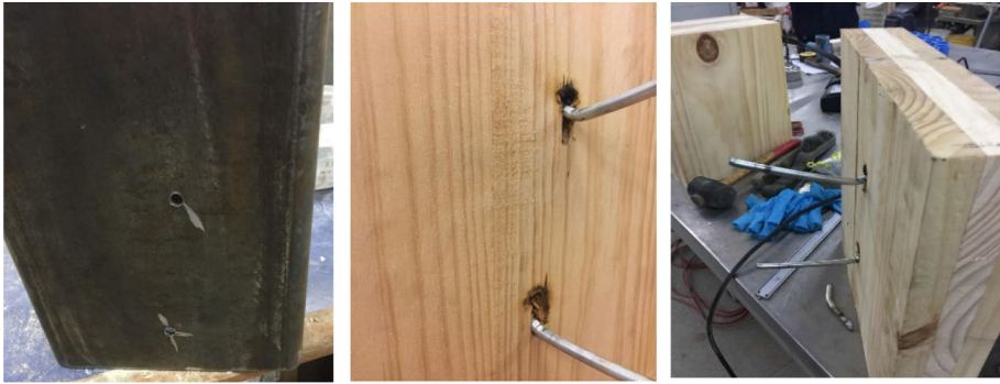
Fig. 3 Ductile failure after fatigue of the dowels in the CLT-steel connection (Carrero et al. 2020)
