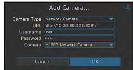
Fig. 11. Adding local cameras or network cameras.
