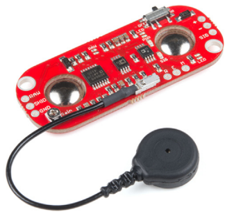
Fig. 8. Arduino-powered, all-in-one electromyography (EMG) sensor from Advancer Technologies.
