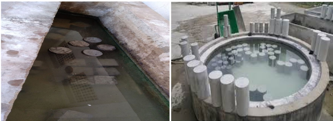
Fig. 10 Water curing of various concrete specimens
