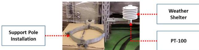
Figure 5 - Ambient temperature sensor shelter.
