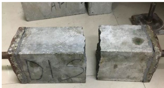
(a) The failure location of specimens
