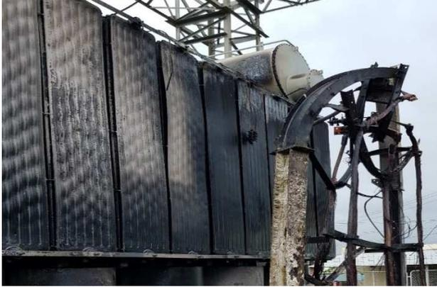
Fig. 9. 120MVA 132/33kV transformer failure in Kushtia substation.
