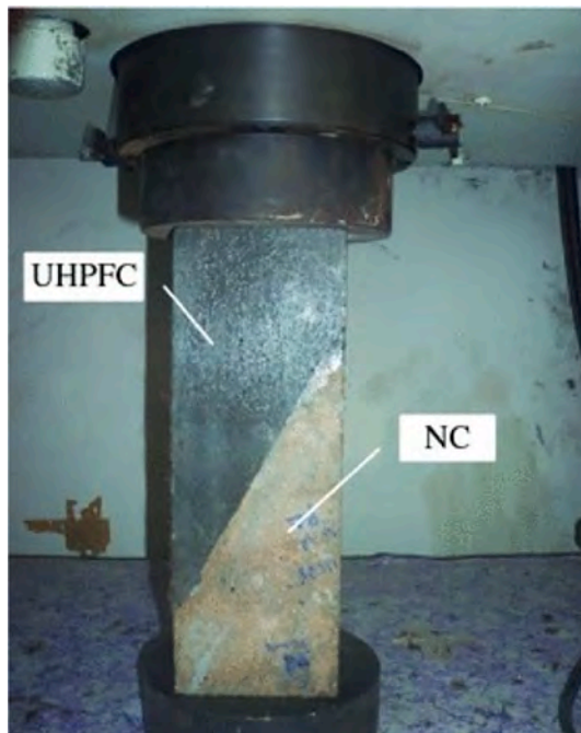
Fig. 12. Slant shear test set-up for UHPC-NC specimen [89].
