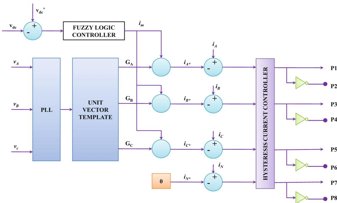
Fig. 2 Circuit representation of grid interfacing control using Fuzzy PI controller
