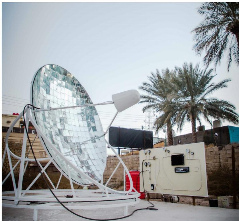
Fig. 2. Parabolic solar dish–steam power plant system.
