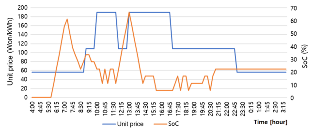
Fig. 13 Hourly unit prices and SoC changes on the days when peak power demand occurred
