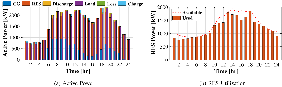
Fig. 11. Active power balance and RES utilization for case II with 3 hour droop time frame.
