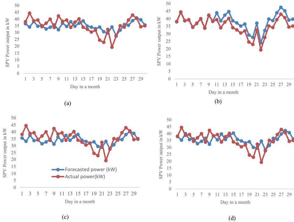
**Figure 7.** Comparison of actual PV power (kW) output with forecasted PV power (kW) output.
