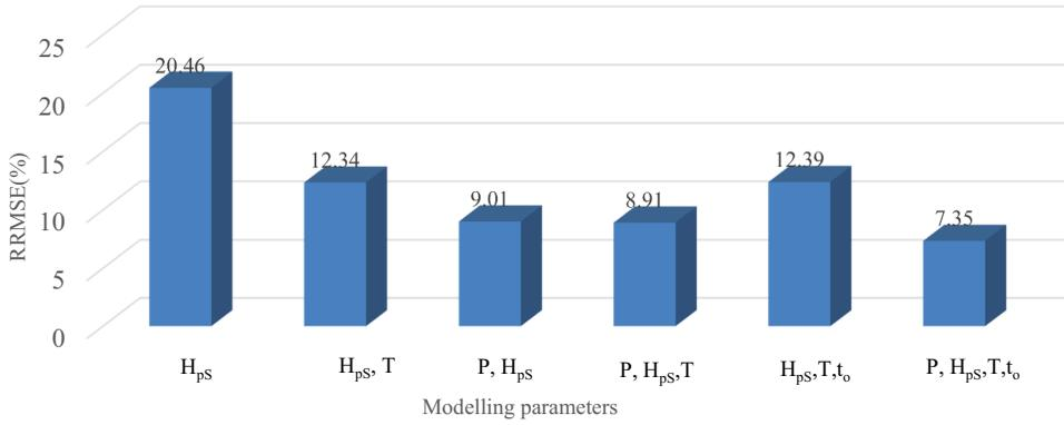
Figure 5. Performance of hybrid-ANN forecaster-S with different inputs and combination of inputs.
