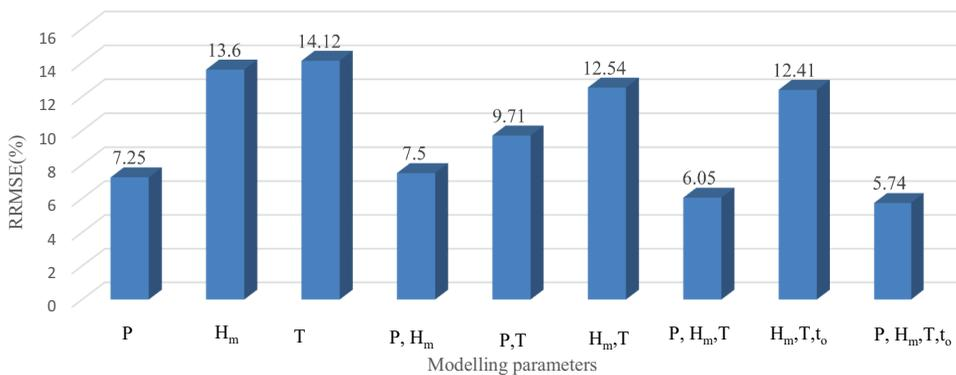
**Figure 4.** Performance of ANN forecaster with different inputs and combination of input parameters.
