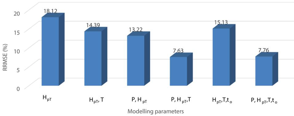
Figure 6. Performance of hybrid-ANN forecaster-T with different inputs and combination of input parameters.
