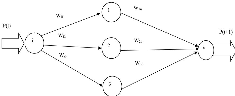
**Figure 1.** A functional diagram of back-propagation multilayer perceptron (BP-MLP) network.
