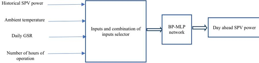
**Figure 2.** ANN forecaster with different inputs and combination of inputs.
