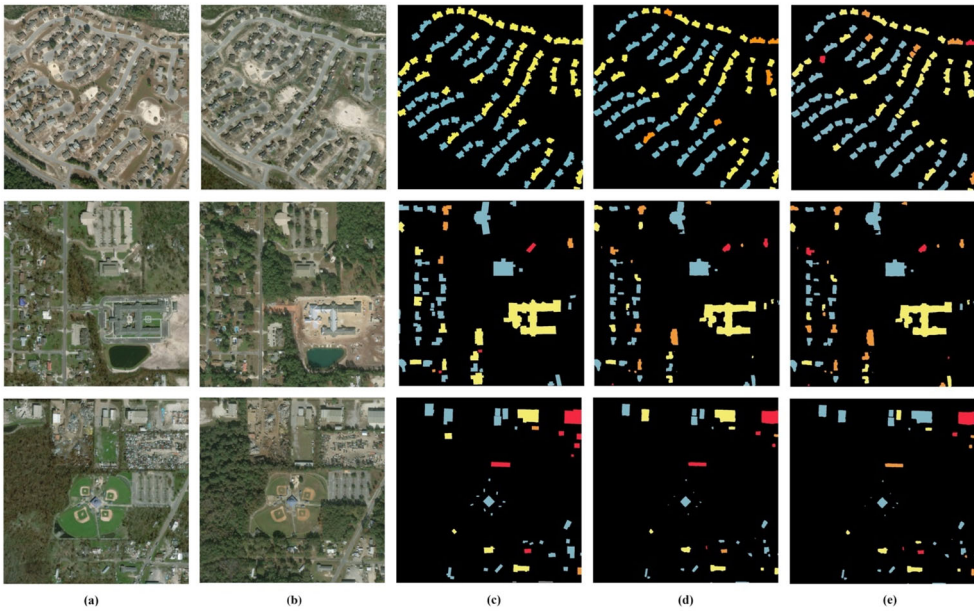
Figure 4. Visual evaluation of the coupled damage assessment model at three localities. (a) Pre-event images, (b) post-event images, (c) annotated buildings and damage classes from the training dataset, (d) segmented buildings with CNN output classes, (e) segmented buildings with SVM output classes. Color legend: blue – undamaged, yellow – minor damage, orange – major damage, red – destroyed buildings.
