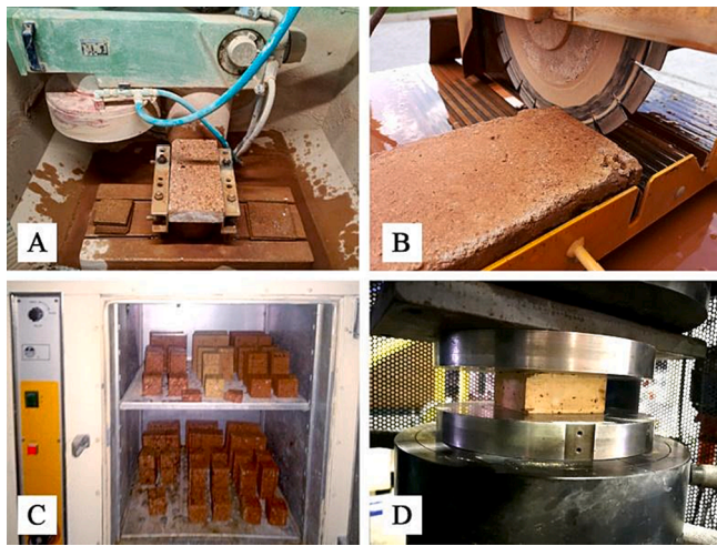
Fig. 4. Manufacturing process of the specimens: (A) the grinder equipped with a rotary disc to polish the bricks until obtaining a constant thickness; (B) the table saw equipped with a water jet to cut the specimens; (C) the specimens in the oven at a constant temperature of 105 \pm 5 \text{ }^\circ\text{C} for 24 hours; (D) 100 \times 100 \times 40 \text{ mm}^3 specimen tested in the hydraulic press.
