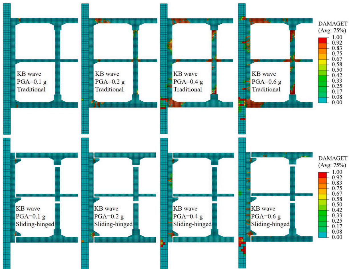
Fig. 15. Tensile damage nephogram of the station with innovative design. KB wave.
