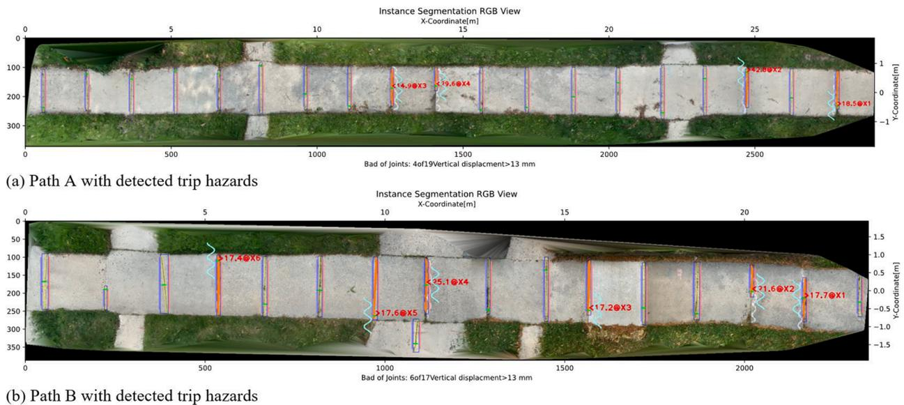
Fig. 12. Experimental results of Paths A and B with trip hazards.
