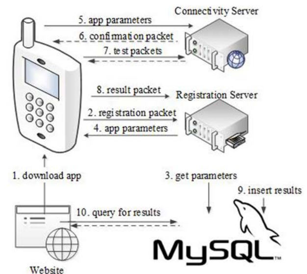
Figure 5: MIST architecture and communication protocol (adapted from Wittie et al. 2007).
