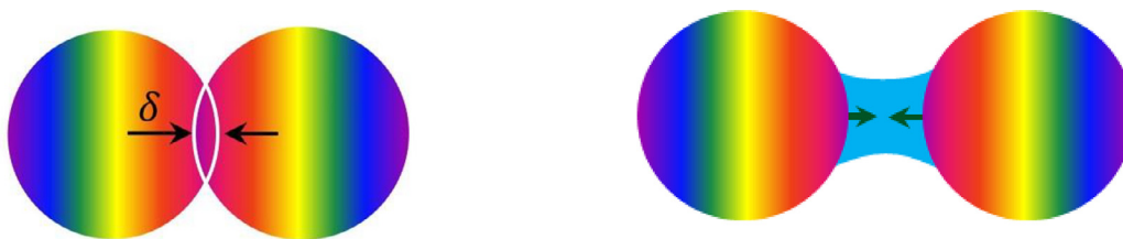
Fig. 1. Exhibition of repulsive force due to physical contact and existence of attraction force due to the moisture cohesion.
