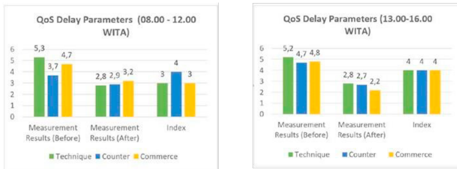
Fig. 6. (a) QoS Delay Parameters during Rush Hours; (b) QoS Delay Parameters during Normal Hours.
